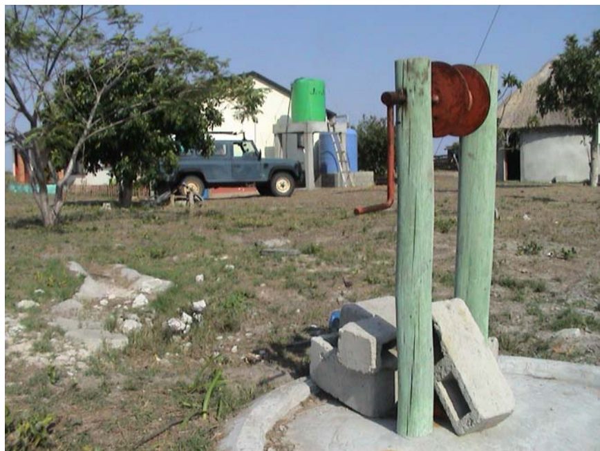
Figure 8: Upgraded Bucket pump
