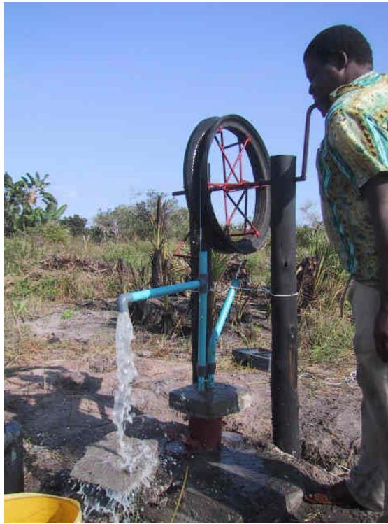
Figure 9: Newly installed rope and washer pump
