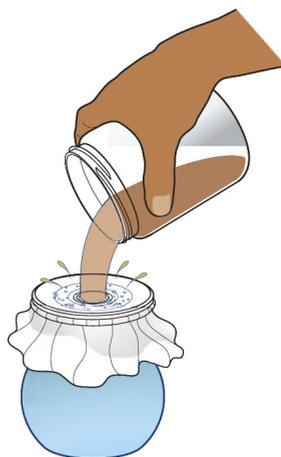
**Figure 33.** Straining water through a fine mesh cloth
