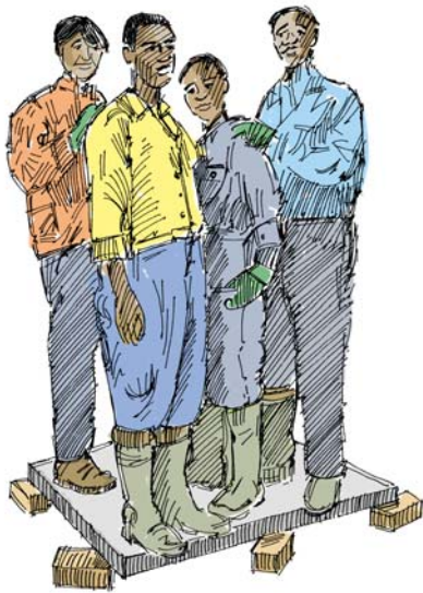
Figure 27. Testing the slab
