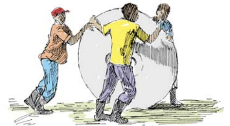
Figure 6. Circular slabs can be rolled into position, making them easier to move over short distances
