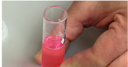
**Figure 9.** Water with a high concentration of chlorine
