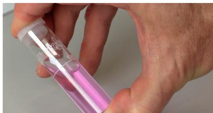
**Figure 14.** Adding the nitricol tablet will cause the colour to change
