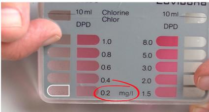
**Figure 8.** Water with a low concentration of chlorine
