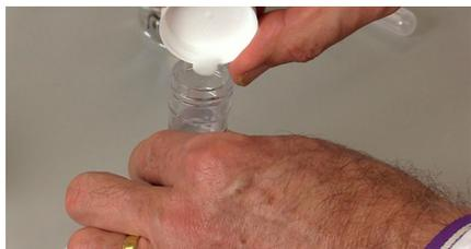
**Figure 13.** Adding the nitrate test tablet
