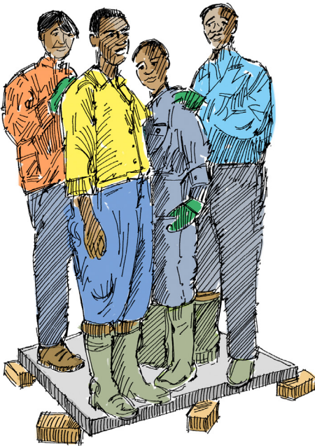
Figure 6. Four men test the strength of a latrine slab
