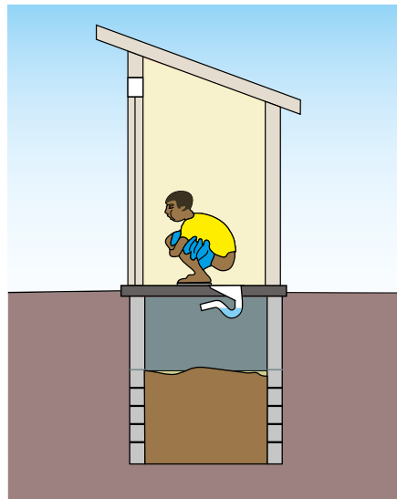
Figure 3. A direct pour-flush latrine
