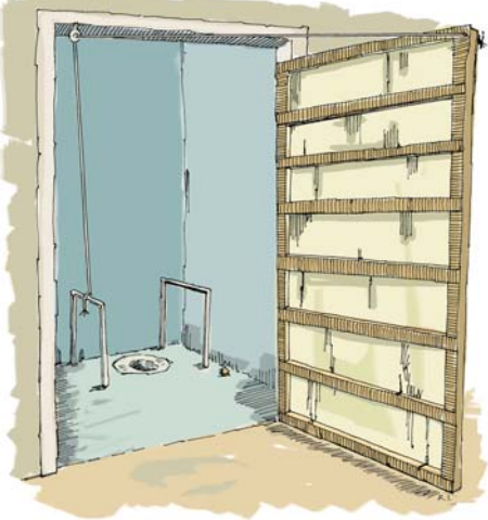
Figure 5. Latrine door closing method for disabled users
