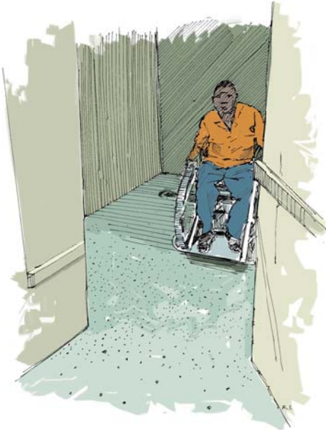
Figure 4. Latrine with a wide opening and enough space for a wheelchair to turn
