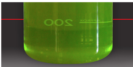
Figure 1. A jar containing fluorescein: light passing through is not scattered
