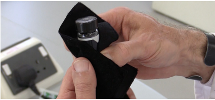
Figure 22. Cleaning the exterior of the tube
