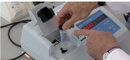
Figure 23. Placing the tube into the turbidity meter
