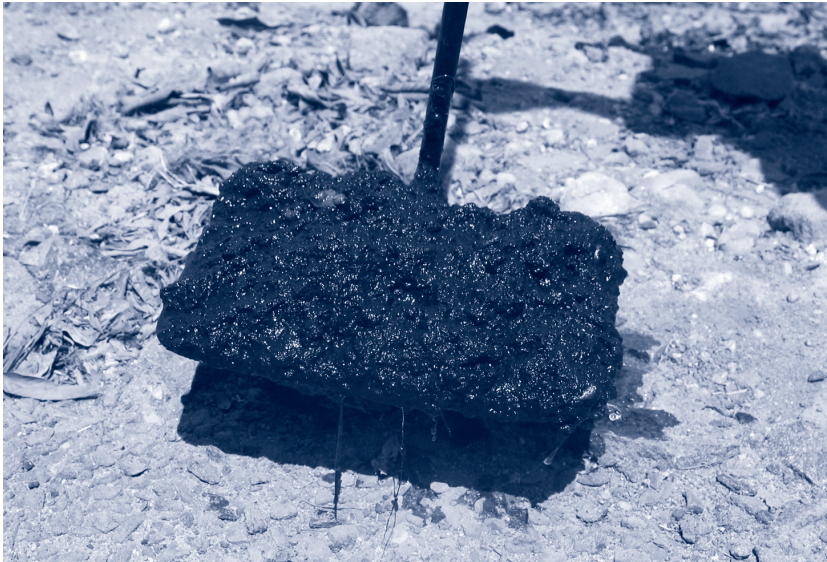
Picture 8.4: Sludge from a septic tank in India – the black colour of the sludge indicates anaerobic condition
