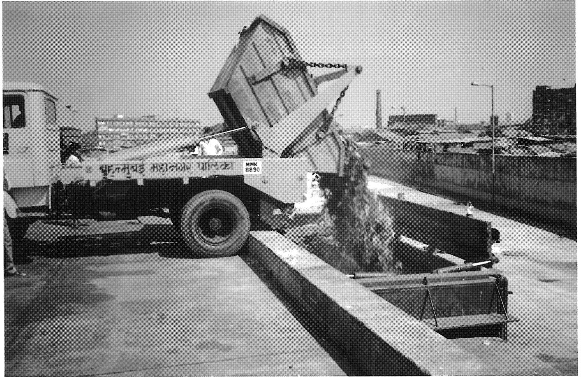
Photograph 4 Transfer of waste from a dumper-placer into a bulk refuse carrier at Mahalaxmi transfer station, Mumbai
