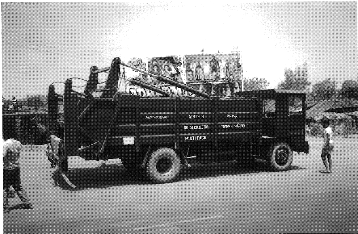
Photograph 6 A Multipack compactor truck, similar to those widely used for collecting solid waste in Mumbai. Chapter B-2 discusses the operation of these trucks and Chapter D gives some information about their maintenance
