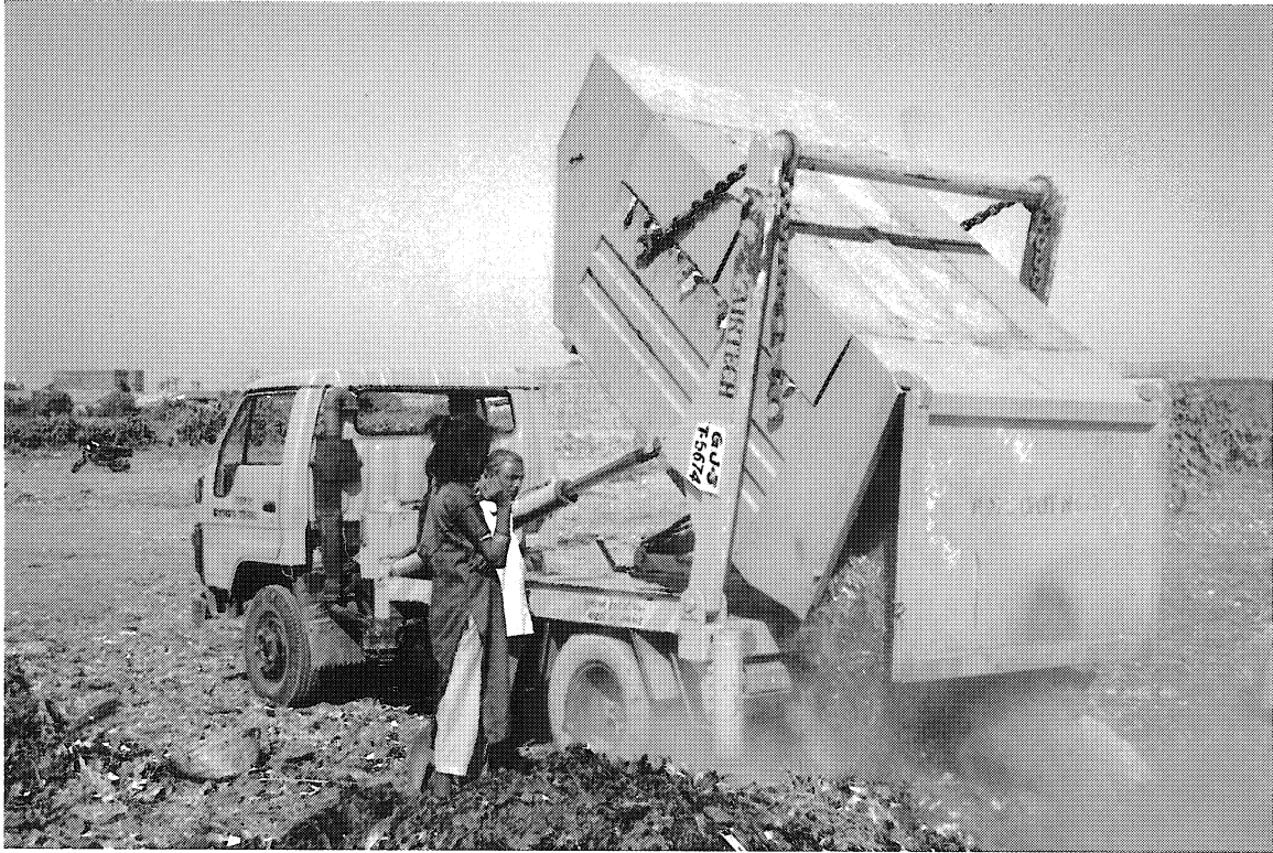
Photograph 8 Municipal dumper-placer vehicle unloading at Rajkot (Chapter B-3)
