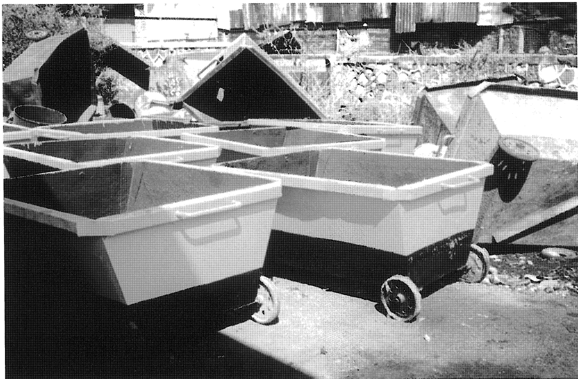
Photograph 7 Trolley bins (or wheeled containers) for use in conjunction with compactor trucks. In the foreground are bins that have been overhauled; in the background are containers awaiting repair (Chapter B-2)
