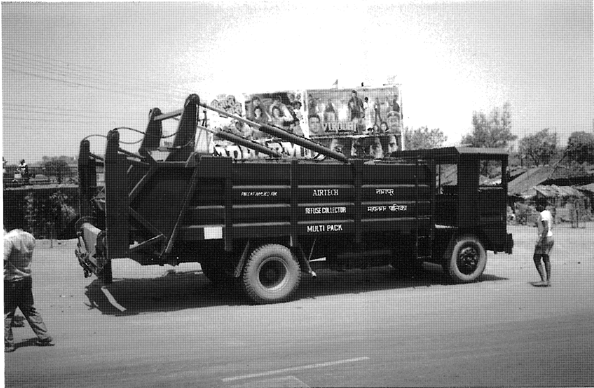
Photograph 6 A Multipack compactor truck, similar to those widely used for collecting solid waste in Mumbai. Chapter B-2 discusses the operation of these trucks and Chapter D gives some information about their maintenance
