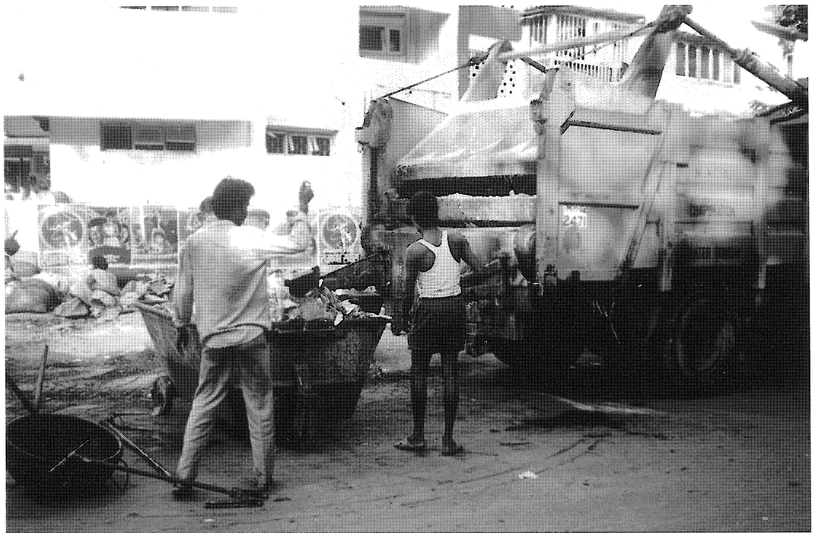
Photograph 5 A Multipack compactor truck preparing to empty a trolley bin in the suburbs of Mumbai. Note the loaders' tools on the left. (Chapter B-2)
