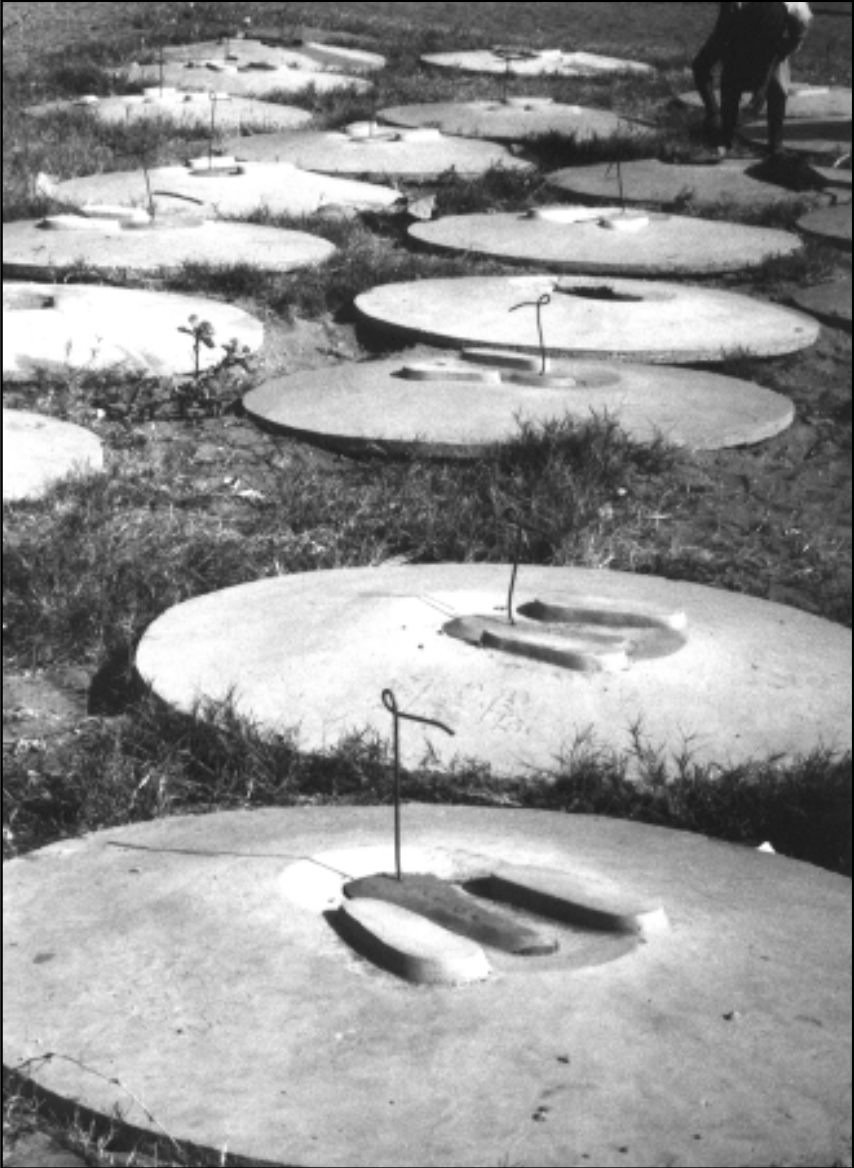
Photograph 3: Production of popular unreinforced domed slabs used for low cost simple pit latrines in peri-urban areas of Mozambique
