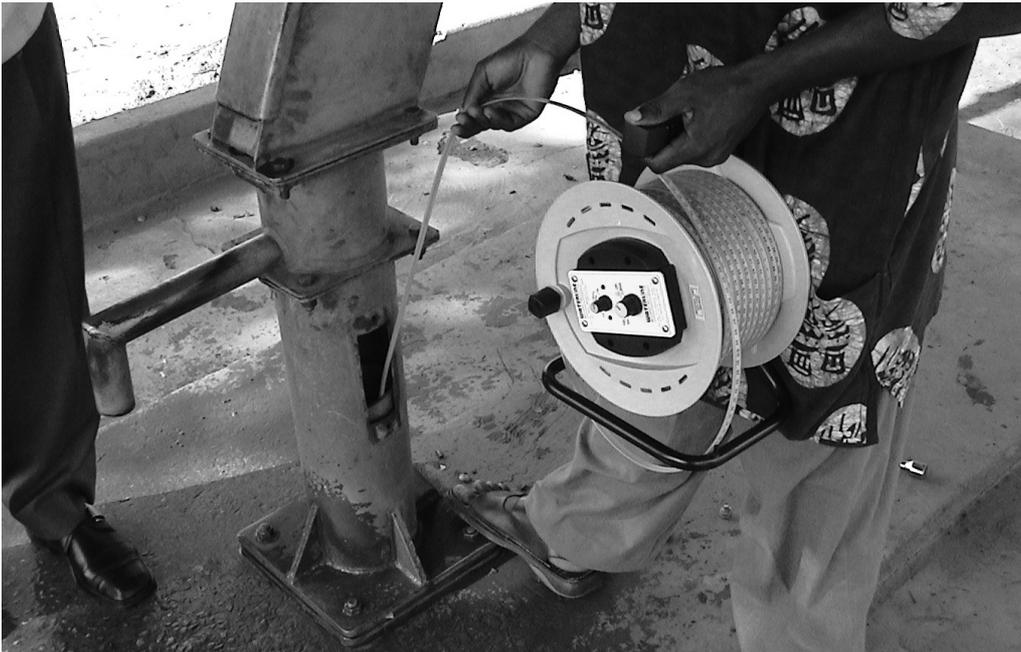
*Photograph 9.1. Monitoring groundwater levels in Ghana*
