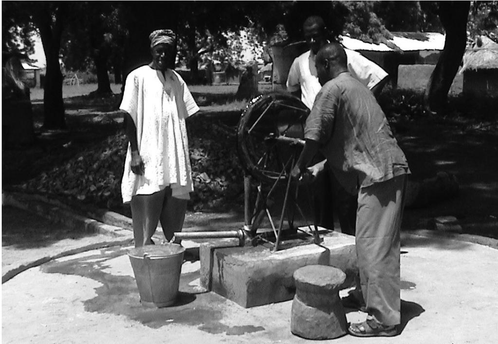
Photograph 6.6. Rope pump on hand-dug well
