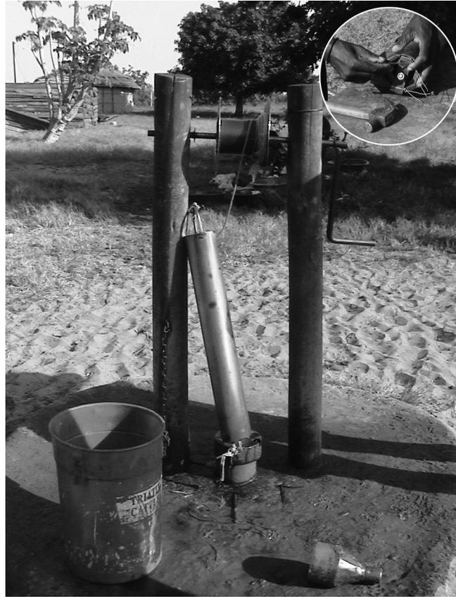
*Photograph 6.7. Bucket pump on tubewell, and undergoing repair*
