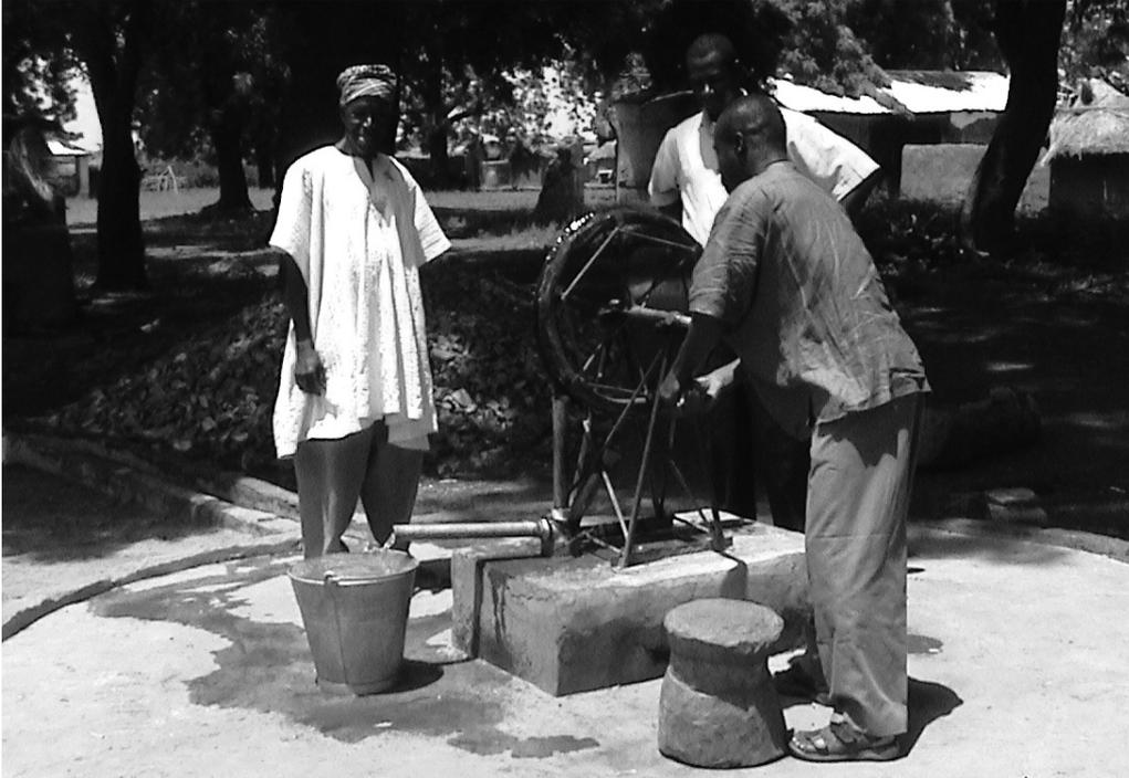
Photograph 6.6. Rope pump on hand-dug well
