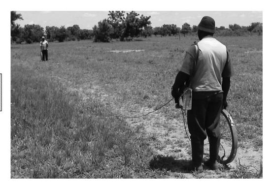
Photograph 6.2. Electromagnetic survey to locate water-bearing fractures
