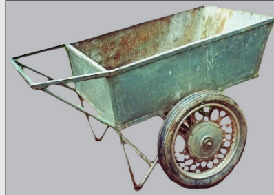
Simple handcart with motorcycle wheels, Lusaka
