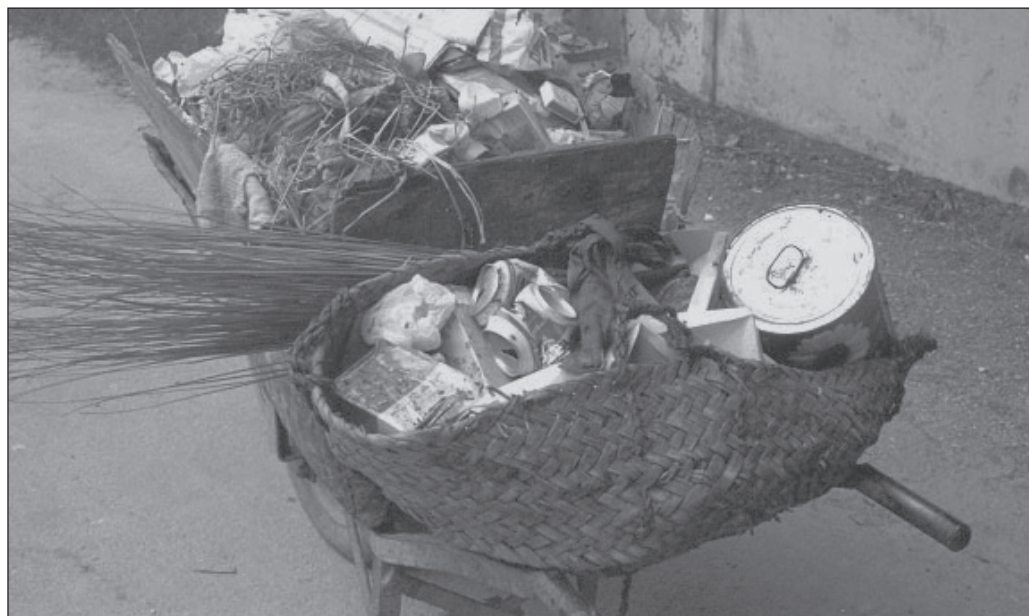
Wheelbarrow adapted for carrying broom and recyclable waste
