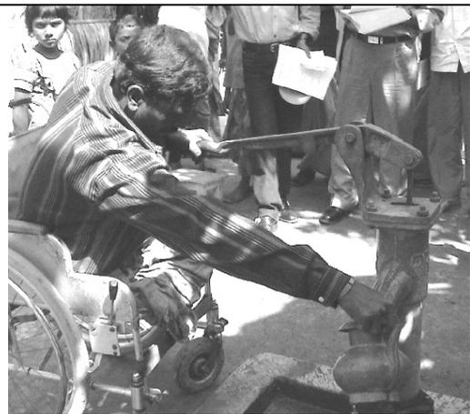
**Fig.2: Wheelchair accessible hand-pump.**
