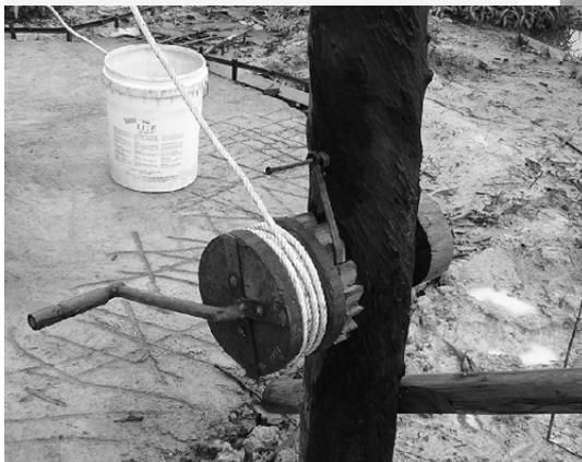
**Figure 5. Ratchet and pawl mechanism, constructed out of wood by Mr Ath.**
