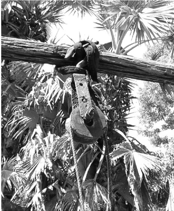
**Figure 3. Hook and pulley arrangement that Mr Tu maintains himself.**
