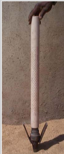
Photograph 9.1. Round aperture well-point
