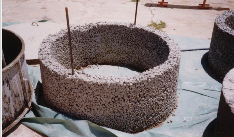
Photograph 5.3. No fines concrete well-screen
