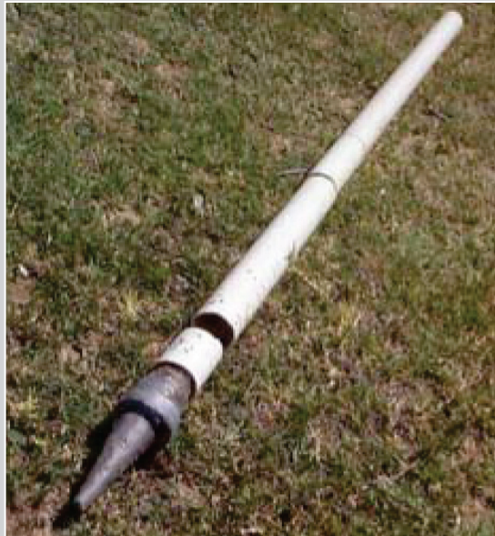
Photograph 5.2. Well-point fracture between transverse slots
