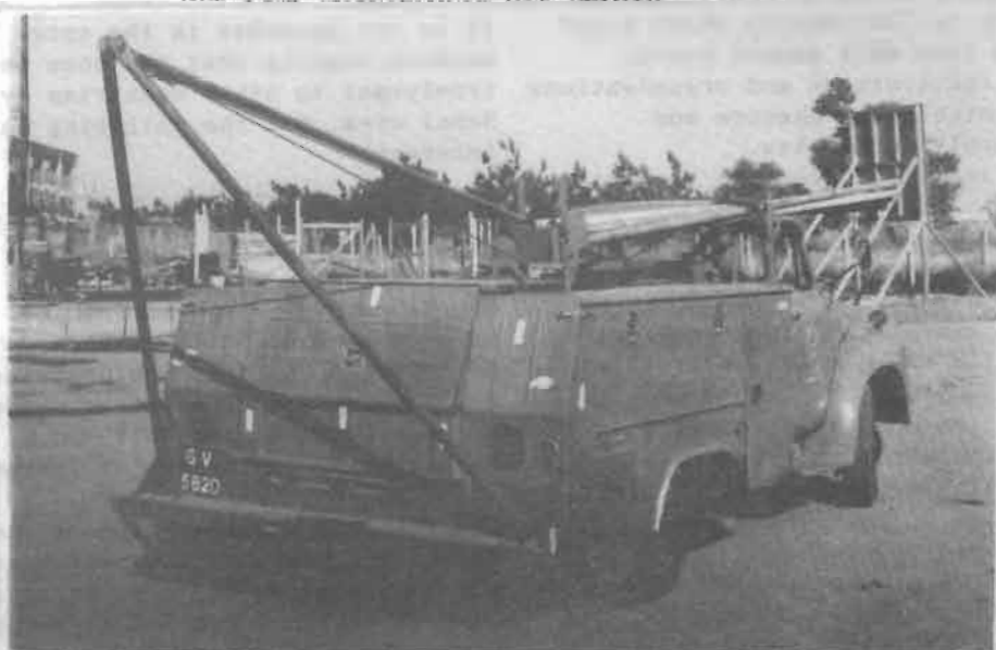
PLATE 3: A SERVICE TRUCK EQUIPPED FOR WELL AND PUMP MAINTENANCE AND REPAIR
