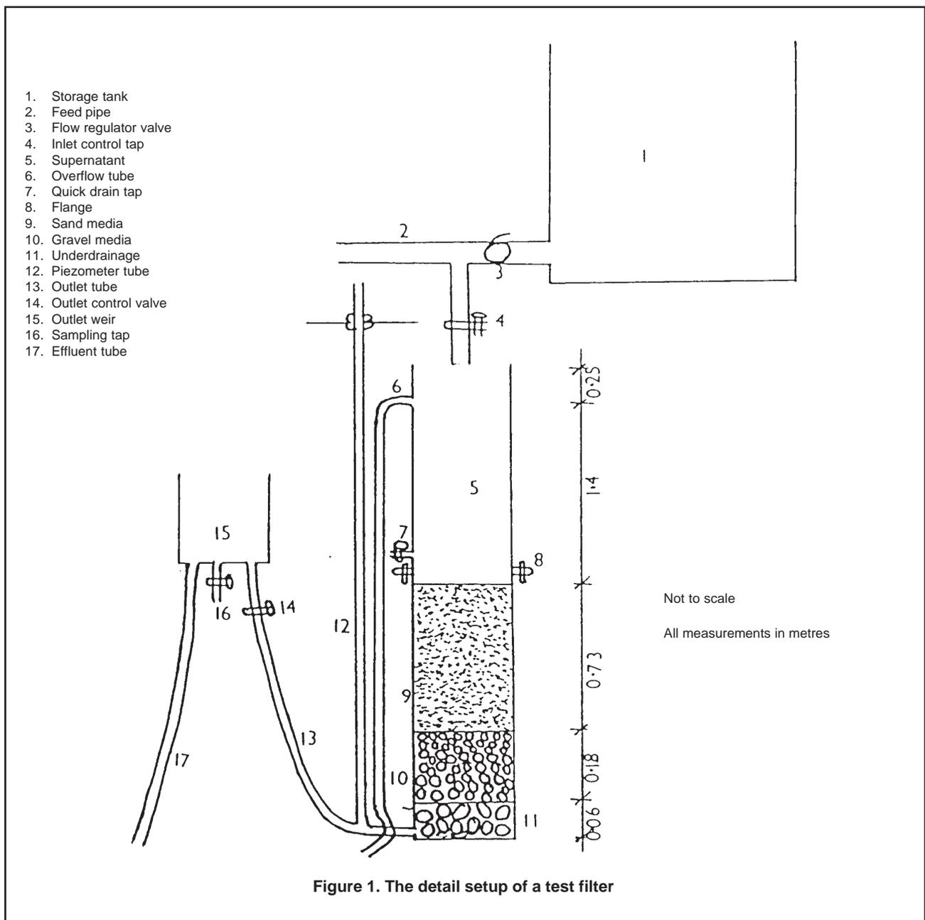
Figure 1. The detail setup of a test filter
