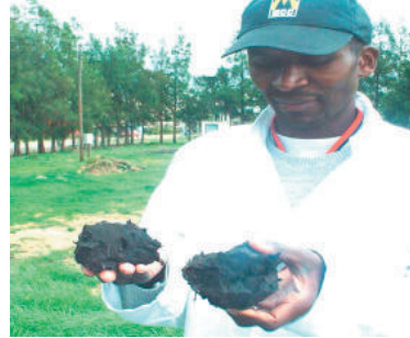
Figure 4. Mud trapped by SSF fabric in Tulbagh
