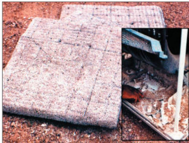
**Photograph 2. Filters from water-based air coolers clogged up with salts (inset: salts accumulating at the base of a cooler)**
