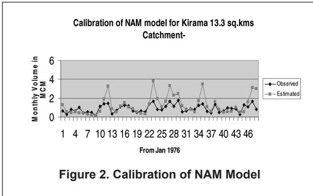
It should be noted that flood peaks are generally underestimated in water balance studies. This is due to the underestimation of spillage. Therefore estimated flood flows by the NAM model are higher than the flow estimated from the water balance study.
