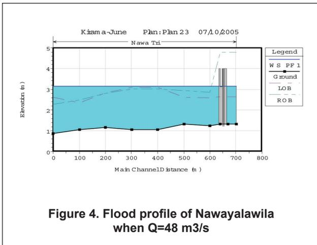
**Figure 4. Flood profile of Nawayalawila when Q=48 m<sup>3</sup>/s**
