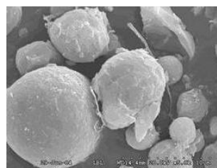
Photograph 2. Scanning electron micrograph of ARUBA (bottom ash coated with iron (hydr)oxides), magnified 5,000x
