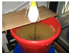
Photograph 4. ARUBA particle suspension with a mechanical mixer
