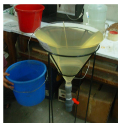
Photograph 5. 10 L/h prototype clarifier being tested at BUET in Summer 2008
