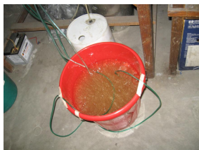
Photograph 3. ARUBA particle suspension through aeration
