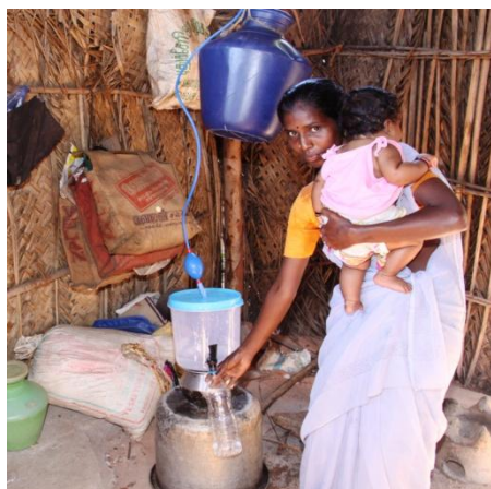
Photograph 7. A Tulip siphon filter. Filter capacity 80 l/ day Life time of element 3000- 7000 litres Retail price 10-14 US$
