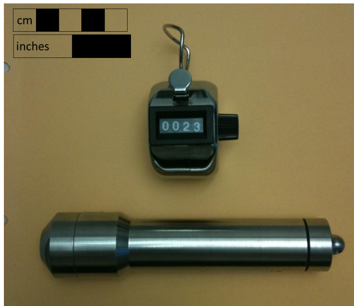
Photograph 1. Tally counter and datalogger
