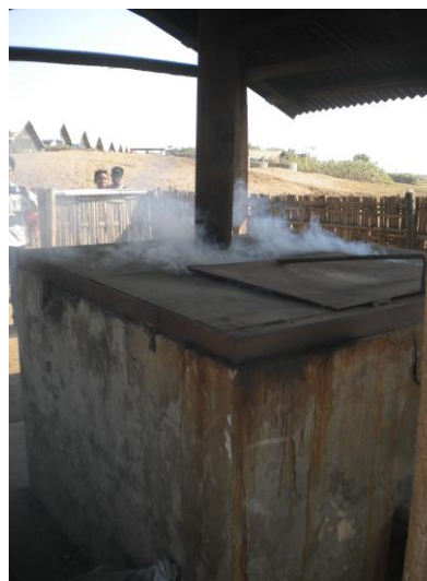
Photograph 2. Malfunctioning two-chamber incinerator used in one of the IDP camps
