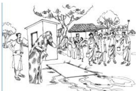
Figure 1. Status of Leach pit in rainy season where water table is high
