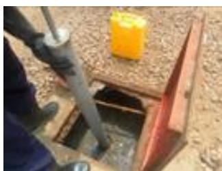
Photograph 1. Picking a faecal sludge sample from septic tank
