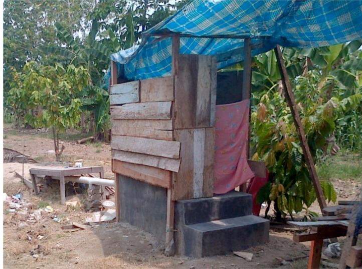
**Figure 2. Example of an elevated latrine built in flood prone areas in Luwu Utara**
