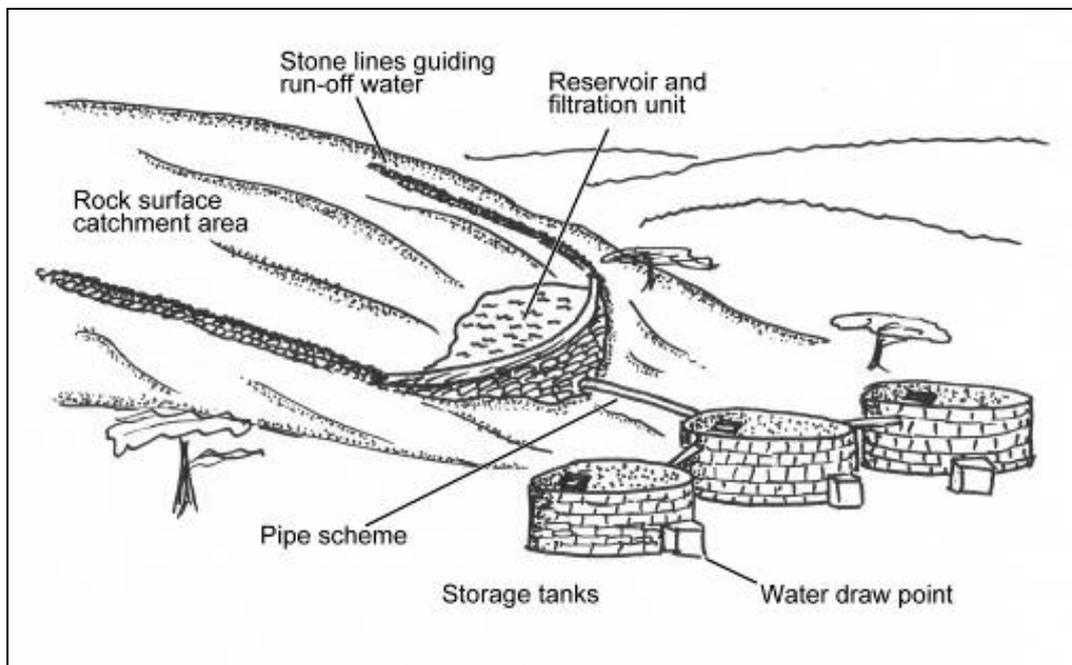
**Figure 2: Schematic representation of a rock catchment system**
