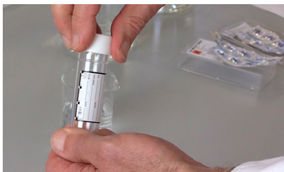
Figure 11. A screw top bottle for testing samples containing nitrate
