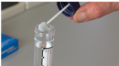
Figure 12. Adding the nitrate powder
