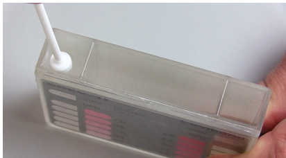
Figure 6. Crushing the tablet
