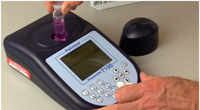
Figure 15. Inserting the test tube into the photometer
