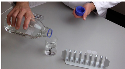
Figure 19. A sample of water suspected of containing a small amount of dissolved iron
