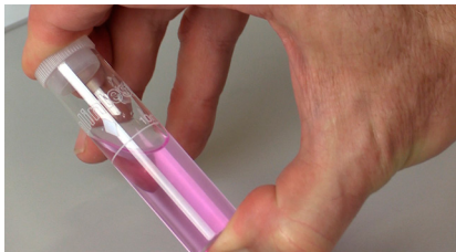
Figure 14. Adding the nitricol tablet will cause the colour to change
