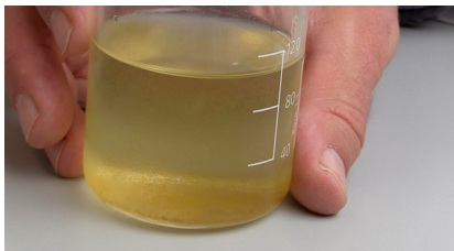
Figure 18. A sample of water containing iron
