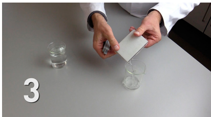
Figure 4. Rinsing out the comparator
