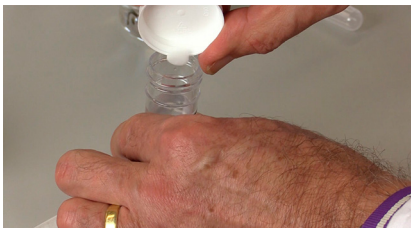
Figure 13. Adding the nitrate test tablet
