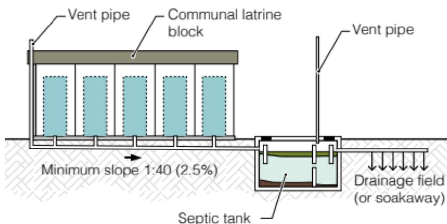
**Figure 2.** Communal toilet connected to a septic tank and drainage field
