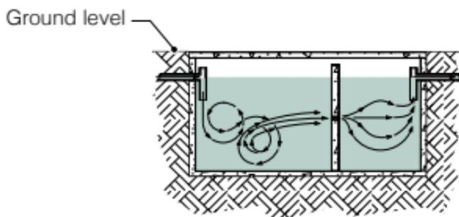
**Small tank – turbulence takes up a large proportion of the first tank**
