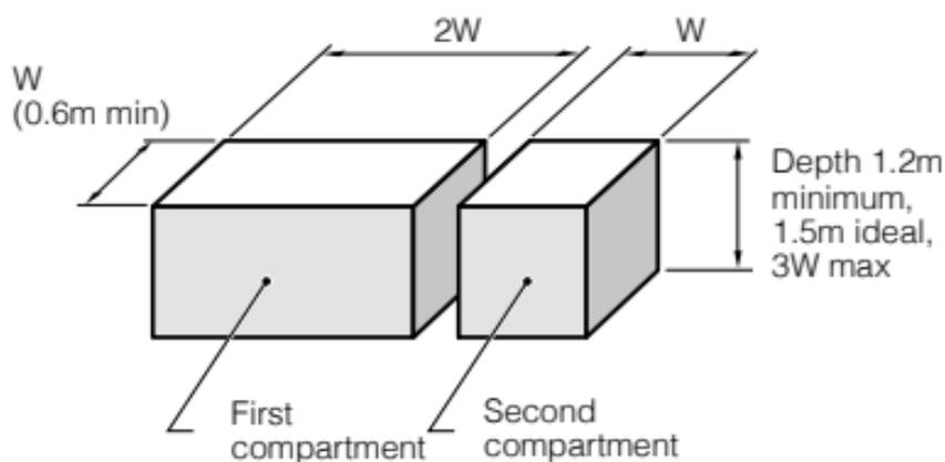
**Figure 7.** Tank dimensions for liquid, scum and sludge volume
