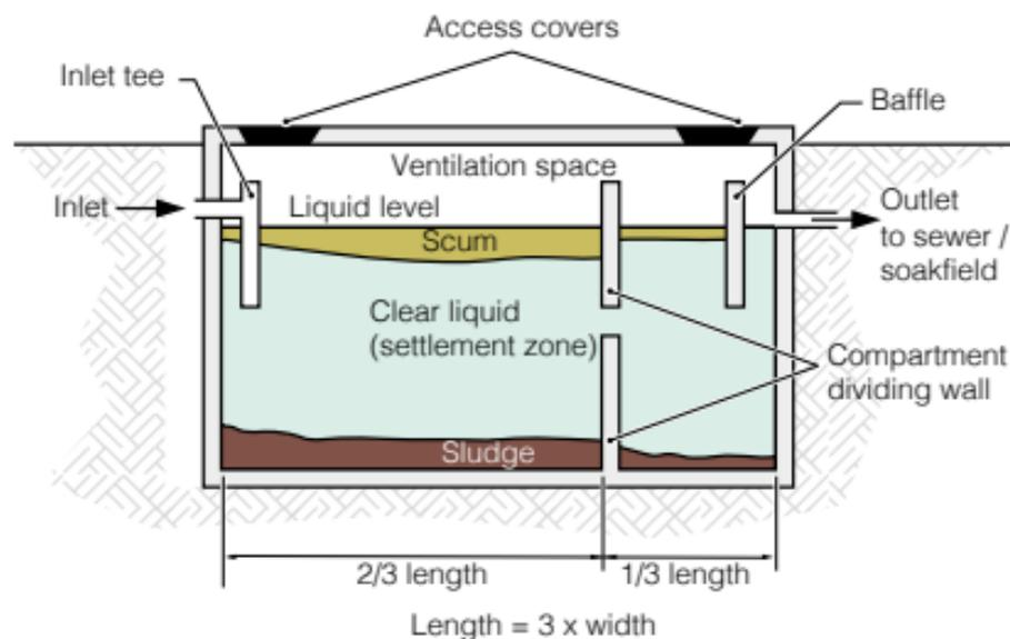
**Figure 5.** Treatment process in a septic tank
