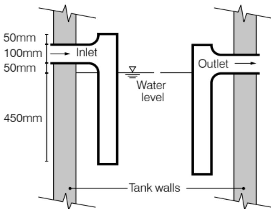
**Figure 8.** Tank inlet and outlet pipes
