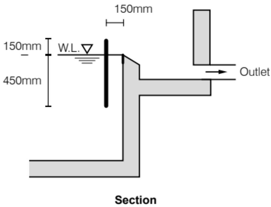
**Figure 9.** Tank outlet using overflow weir
