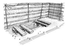
Figure 3. A simple trench latrine: an immediate action to an urgent situation
