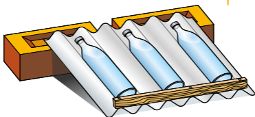
Figure 31. The SODIS system
