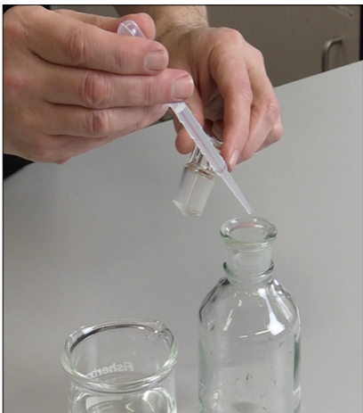
Photo 3. Adding a few drops of aqueous sodium thiosulphate solution
