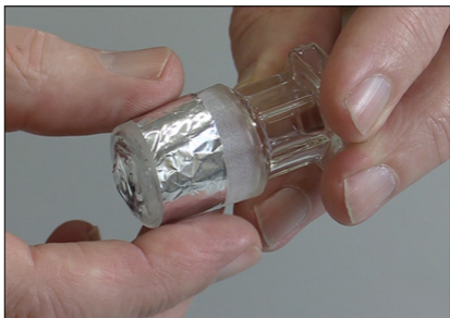
Photo 4. A strip of aluminium foil to prevent the stopper from sticking during sterilization
