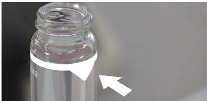
Figure 22. The white triangle should point towards you as you place the tube into the meter
