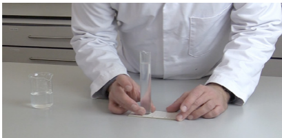
Figure 13. Placing the tube over the panel
