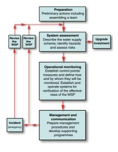
Figure 2. Development and implementation of a water safety plan
