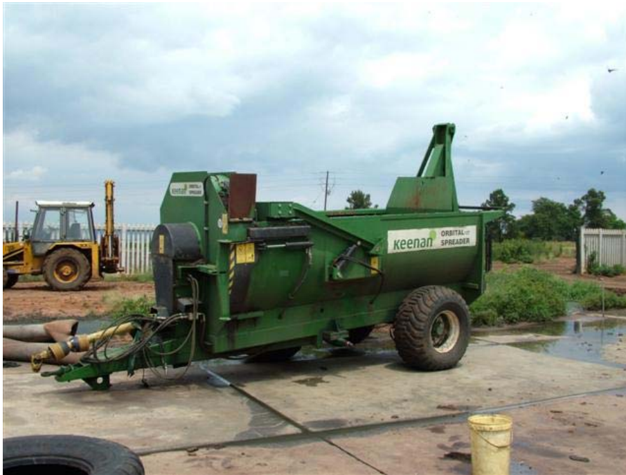
Fig. 38: Cake spreader, re-used silage spreader with wheel missing.
