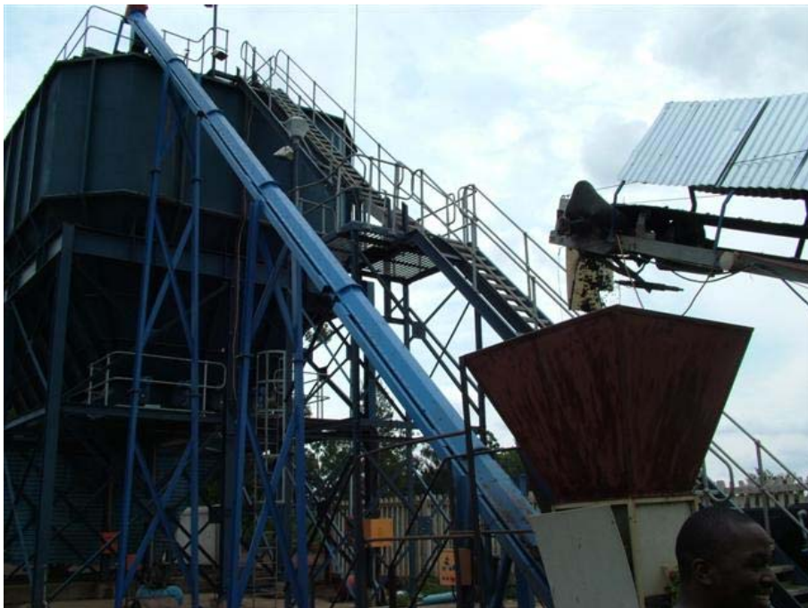
Fig. 37: Inclined cake conveyor transporting cake into elevated hopper.
