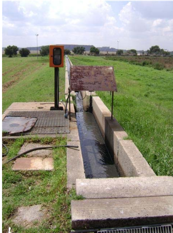
Fig. 69: Flow meter flume and instrument – not set-up or calibrated.
