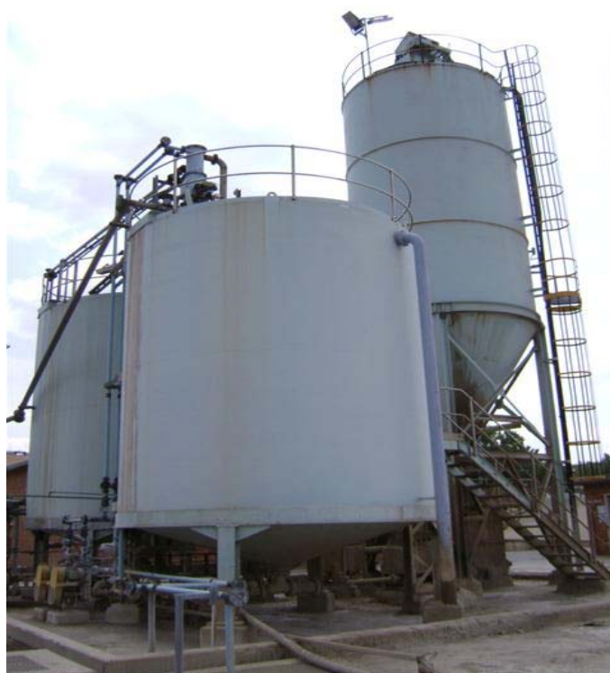
Fig. 50: Slaked lime pH adjustment plant.
