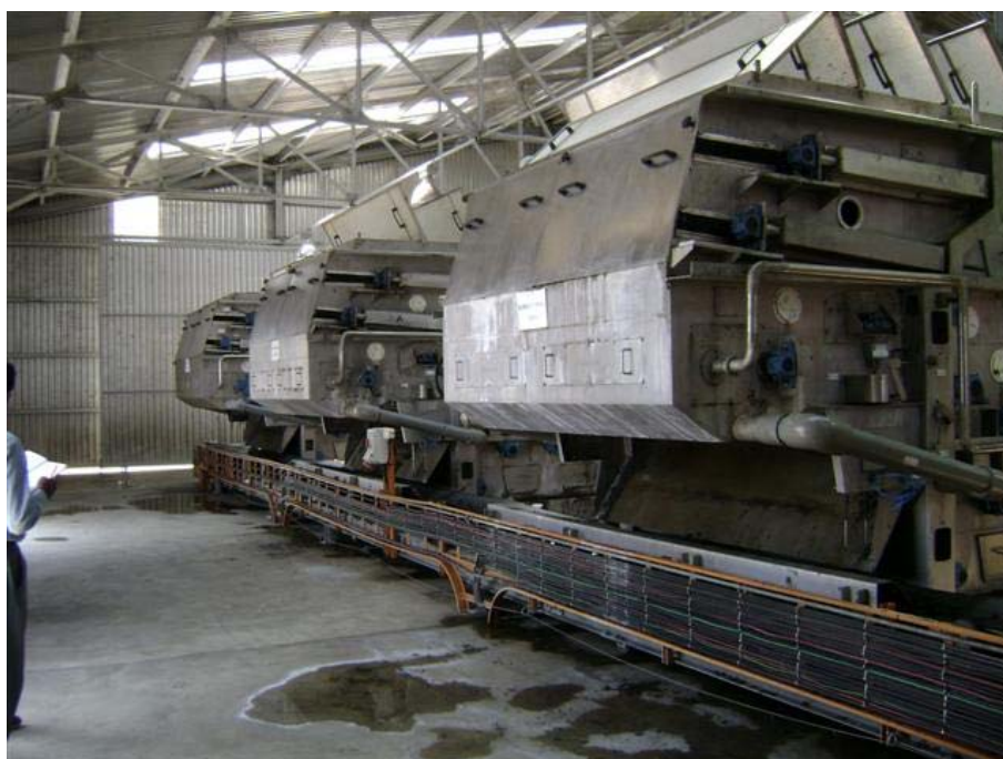
Fig. 47: Sludge dewatering filter presses.
