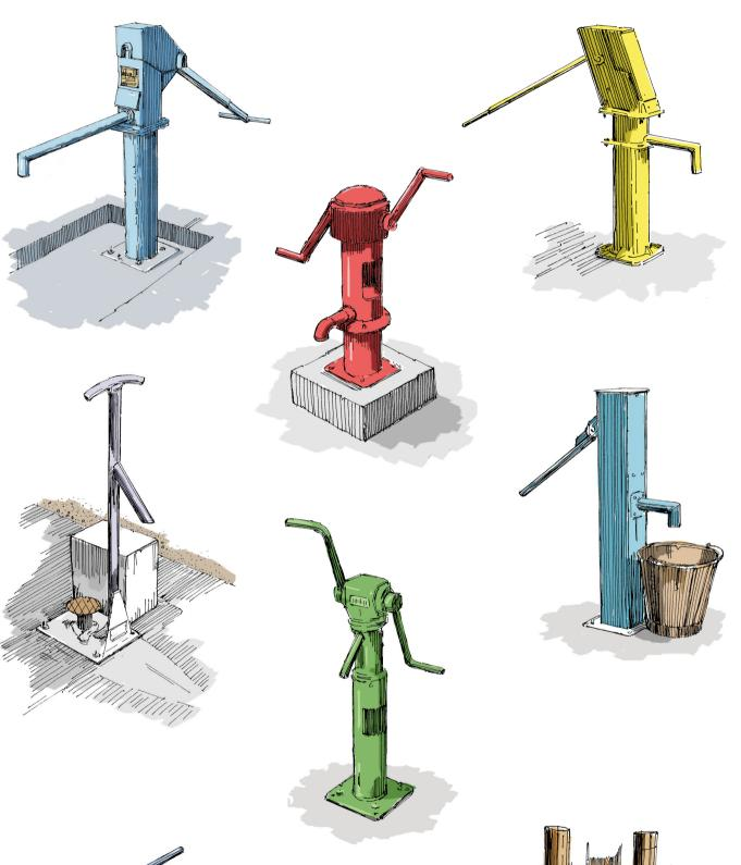
A bucket or other water container is placed under the spout and the user then pumps the water. This may involve pulling on a handle, pushing down on a lever, turning a wheel, winding two handles, pushing down with your foot or even standing on two steps and operating the pump with your legs (so that it is really a foot pump!)
