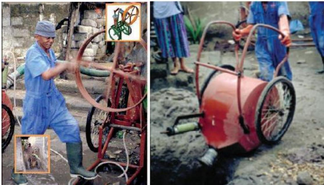
Figure 14 Left: MAPET in use (O'Riordan, 2009); Right: MAPET container being emptied (Thye, et al., 2011)
