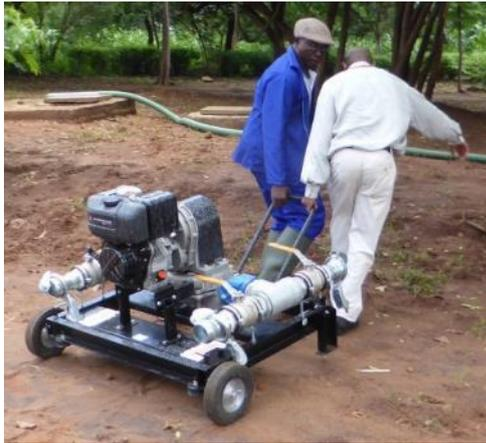
*Figure 5 Diaphragm pump used in Malawi when investigating three pit emptying technologies for 'difficult sludge' (Spit, et al., 2015)*
