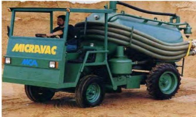
Figure 16 Mircavac – a small scale vacuum technology (Still & O'Riordan, 2012)
