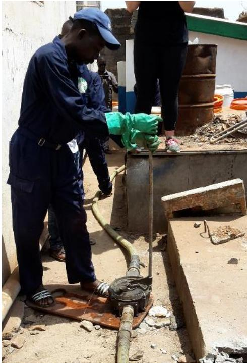
Figure 6 Diaphragm pump used in Freetown (Photo Credit: Mirco Keller)
