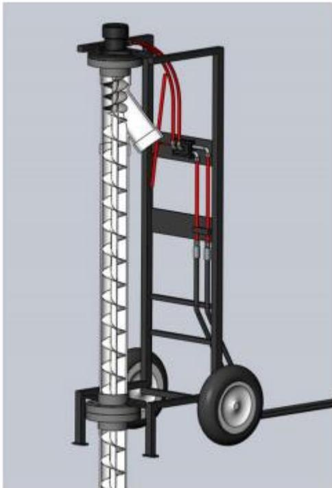
Figure 8 Modified auger - "Excrevator" (Sisco, et al., 2015)
