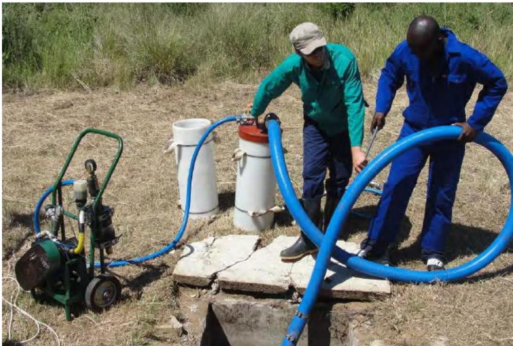
*Figure 15 eVac with two tanks and "suck only" lid fitting (Still & O’Riordan, 2012)*
