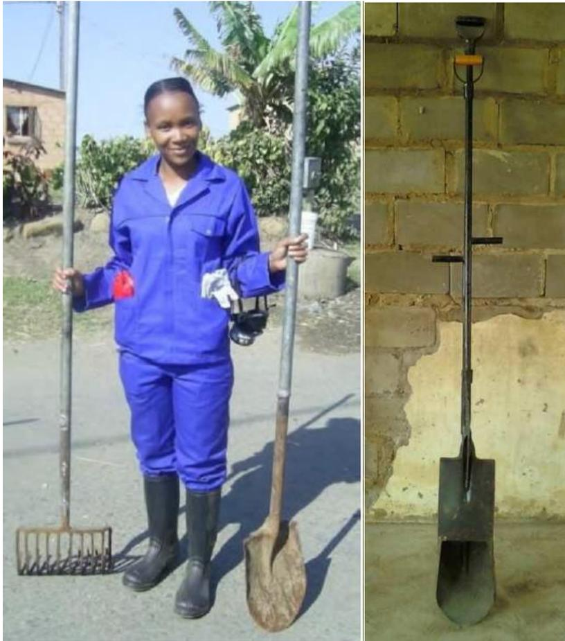
Figure 1 Left: Long handled rake and shovel; Right: Hand shovel/scoop (Still & O'Riordan, 2012)
