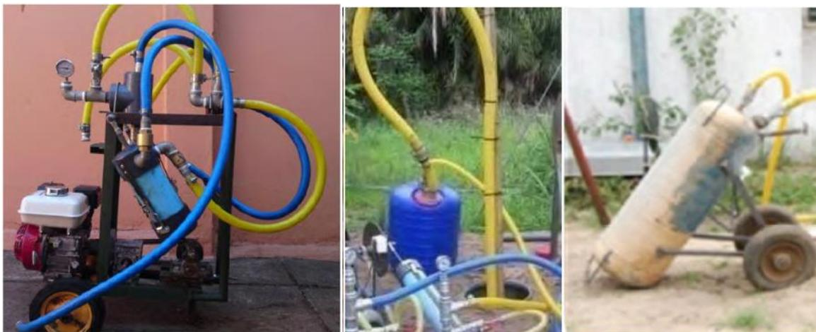
Figure 19 Left: NanoVac prototype; Centre and right: different tanks attachments for the NanoVac (Still & O'Riordan, 2012)
