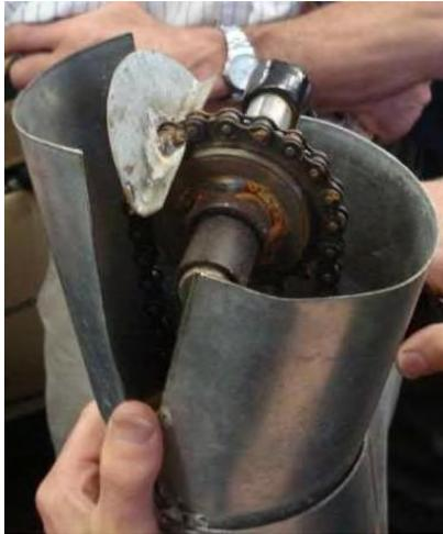
Figure 10 The Nibbler 'scoop' attached to a standard bicycle chain (Still & O'Riordan, 2012; O'Riordan, 2009)
