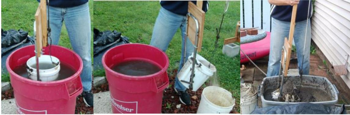
Figure 3 Left and centre: Sludge Digger being used on wet 'sludge'. Right: Sludge Digger used on thick 'sludge'
