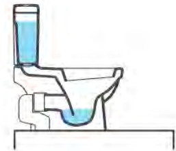
Figure 2.4 – Flush toilet (Tilley et al., 2008)
