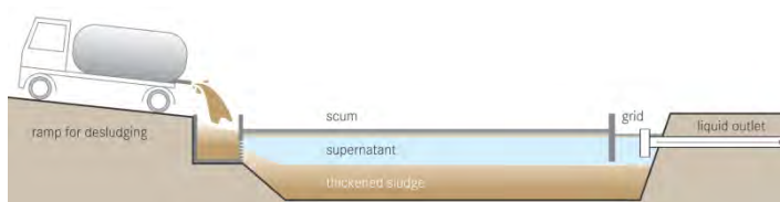
Figure 2.9 – Sludge settling ponds (Tilley et al., 2008)
