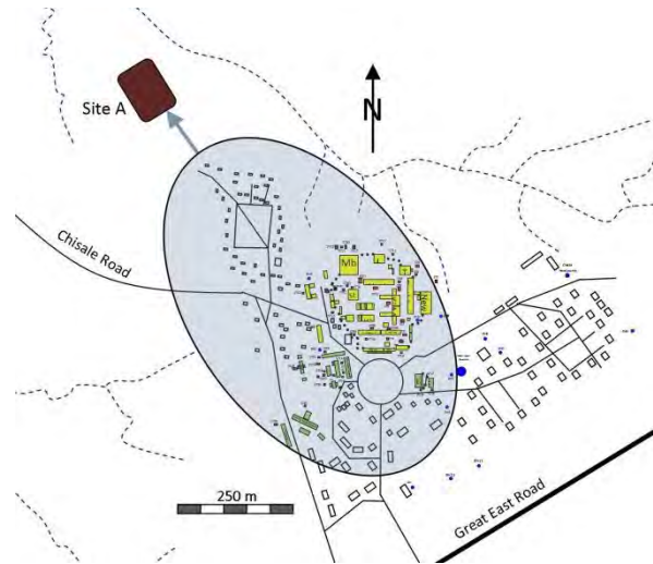
Figure 5.6 – Site A: Location of ponds and approximate coverage area of sewerage system
