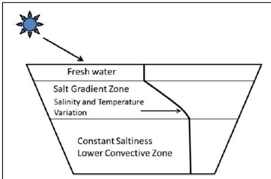
**Figure 31: Typical salt gradient solar pond**
