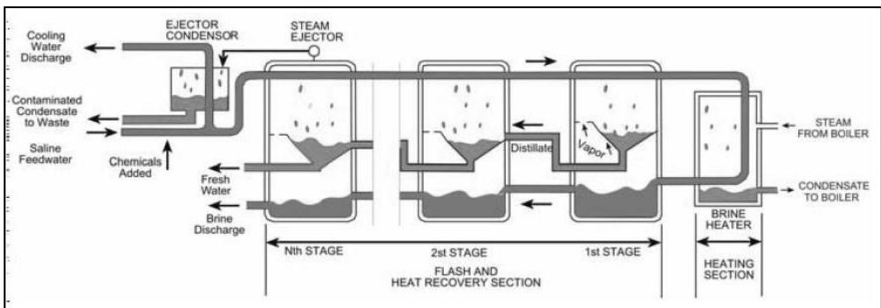
**Figure 14: Simple MSF process scheme**
