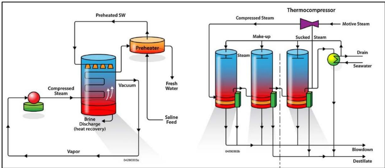
**Figure 16: Diagrams of MVC (left) and TVC (right)**
