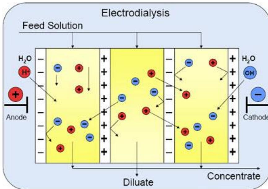
**Figure 19: Electrodialysis simple diagram**
