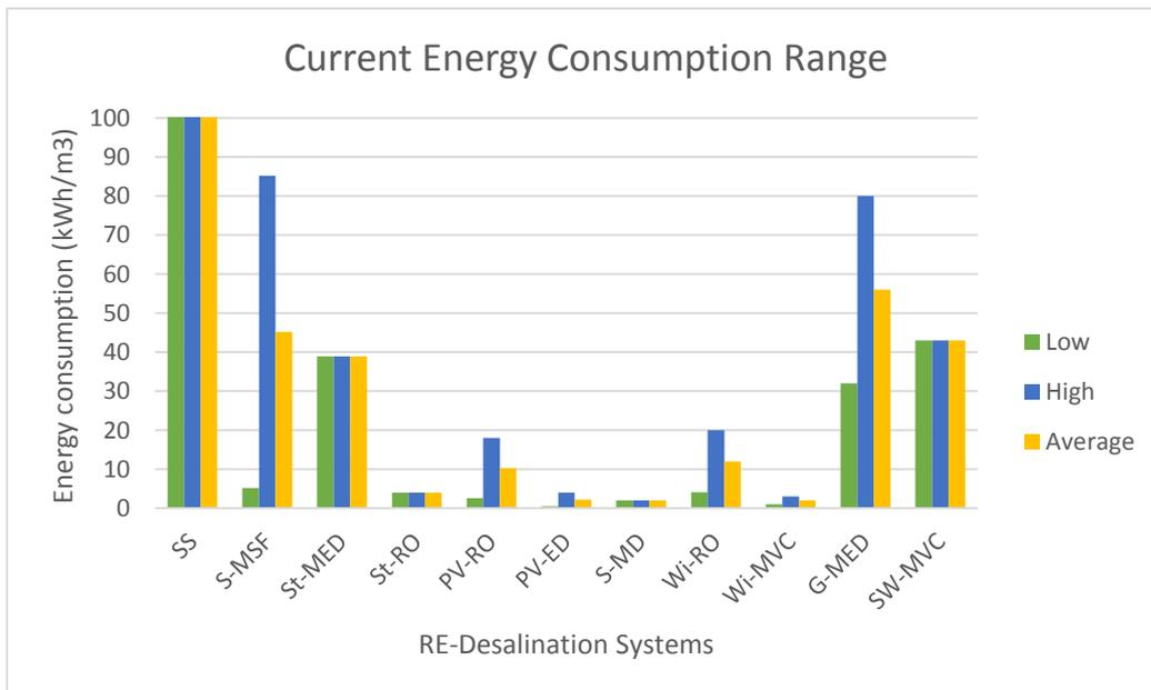
**Figure 42: Current Energy Consumption range of RE-Desalination systems**
