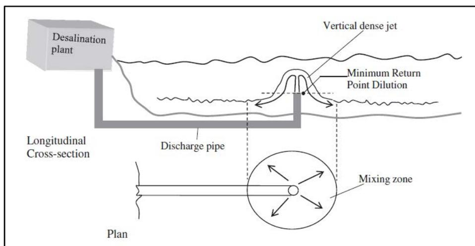
**Figure 33: Simple submerged diffuser discharge**
