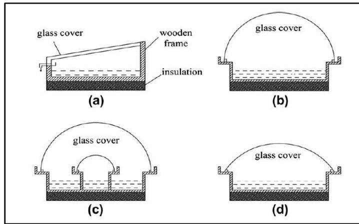
**Figure 36: Basin solar stills with different glass covers**
