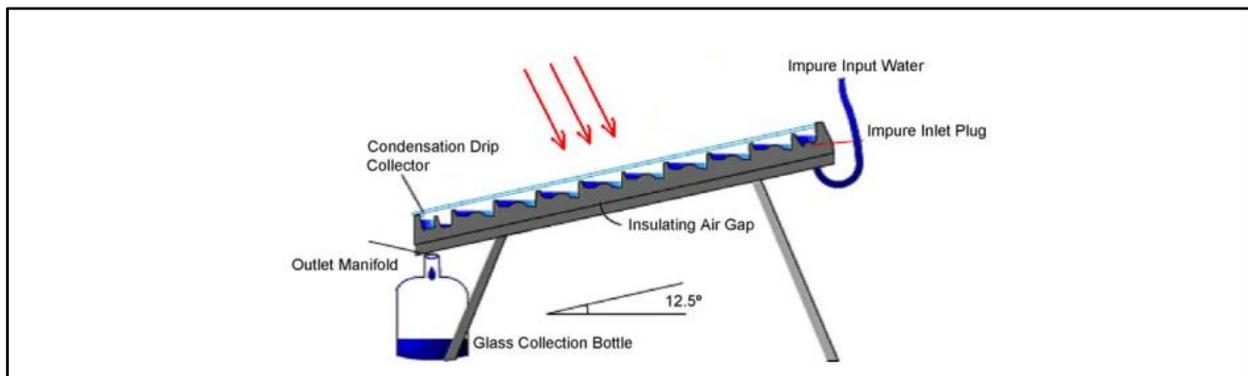
**Figure 22: Schematic diagram of simple solar stills**
