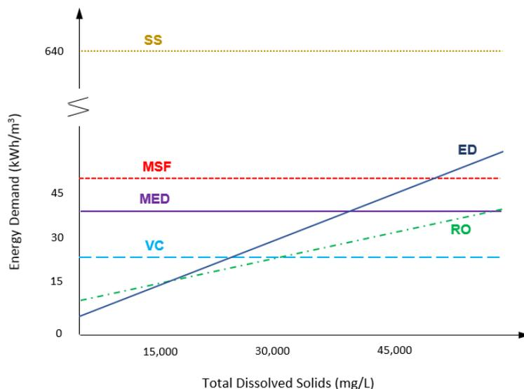
**Figure 25: Salinity vs. Energy Demand for various Desalination methods**
