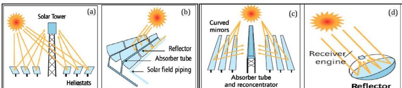
**Figure 28: CSP technologies - a) SPT b) PTC c) LFR d) PDC**
