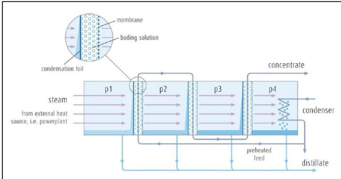
**Figure 21: Schematic of Aquaver MD system**
