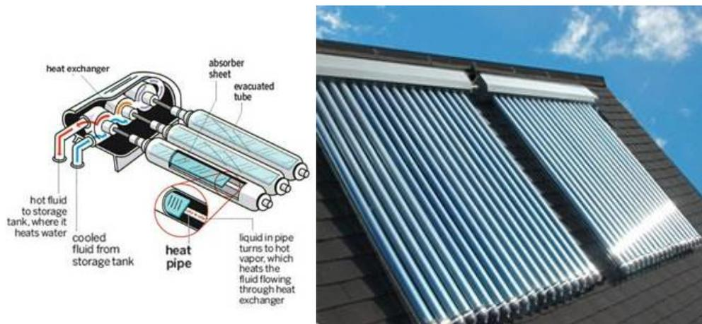
**Figure 32: Evacuated Tube Collectors schematic and image**
