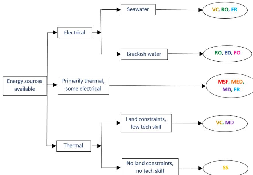
**Figure 24: Selecting a desalination technology**
