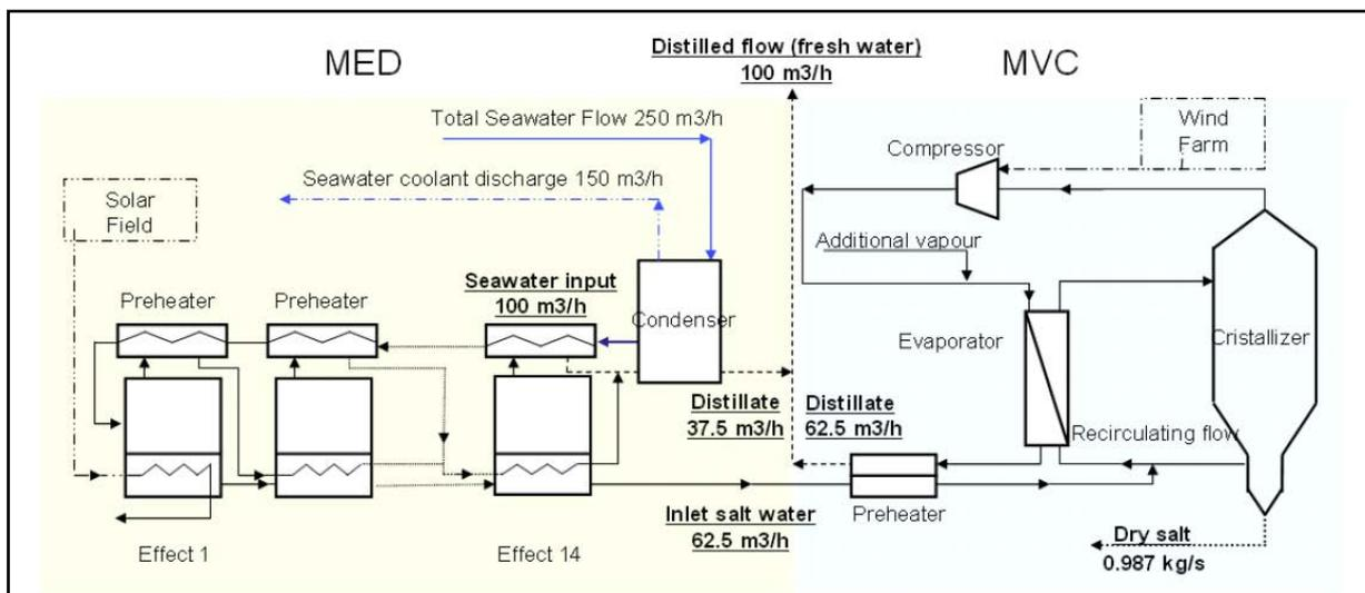
Figure 39: Flow diagram of solar and wind MED-MVC scheme
