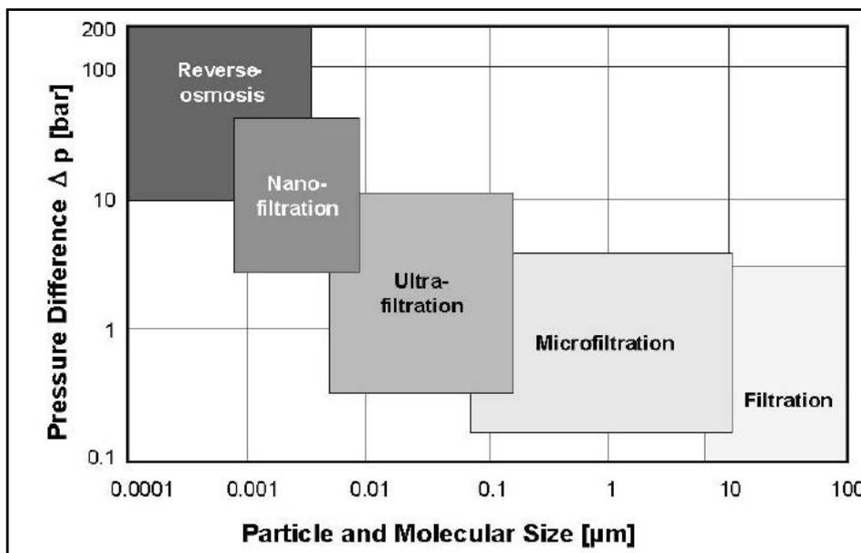
**Figure 23: Separation capabilities of pressure driven membrane separation processes**
