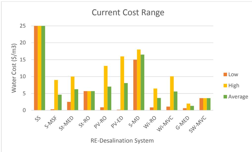
**Figure 41: Current cost range of RE-Desalination systems**
