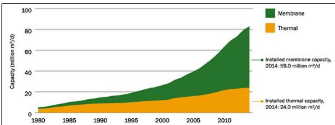
**Figure 12: Cumulative installed membrane and thermal capacity, 1980-2014**
