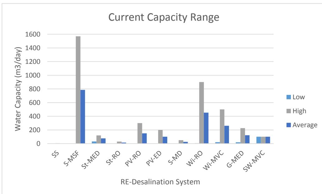
**Figure 40: Current capacity range of RE-Desalination systems**
