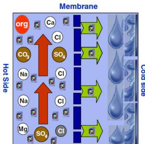
**Figure 20: Membrane Distillation Scheme**
