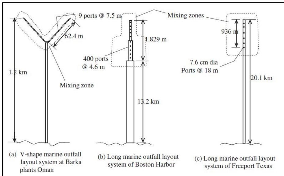
**Figure 34: Various submerged outfall systems**
