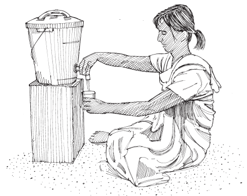
Figure 5.7. Tap fitted to a water bucket
