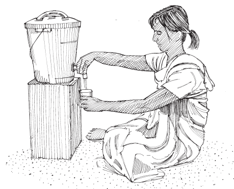
Figure 5.7. Tap fitted to a water bucket
